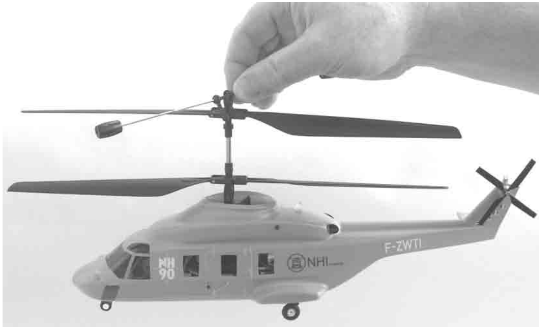
Fig. (8): Suspend the helicopter to balance the machine at C.G.
