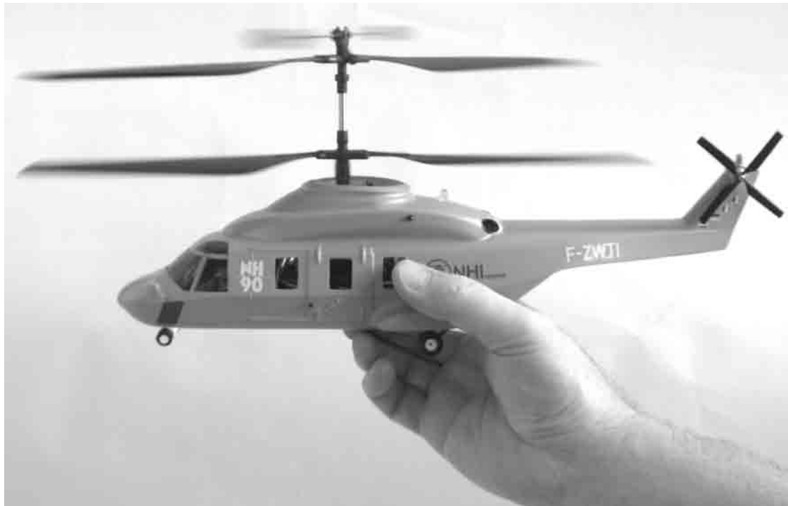
Fig. (14) Hold the helicopter at its C.G.. point
