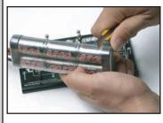
3. Carefully peel off 5 spots with cutter knife where the 5 screws will be tightened.
